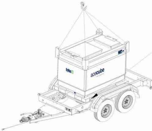
4xM20 GRADE BOLTS, NYLOCK NUTS AND PLAIN WASHERS TO FIX TANK TO AN APPROPRIATE DYNAMIC TRAILER. TRAILER SHOULD HAVE MAX GROSS WEIGHT TO MAX FULLY LADEN CAPACITY AS INDICATED ON THE UN NAME PLATE.
